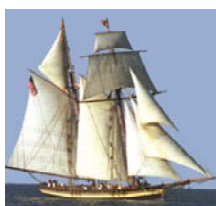
PRIDE OF BALTIMORE, II , Baltimore, Maryland Square topsail schooner, two masted, 170' sparred length, 26' beam, 97 gross tons Owner - Pride of Baltimore, Inc., www.pride2.org
