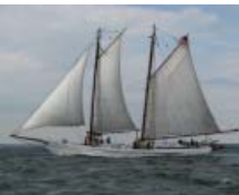
A.J. MEERWALD , Bivalve, New Jersey Two masted Oyster Schooner, 115' sparred length, 22' beam, 57 gross tons Owner- The Bayshore Discovery Project
