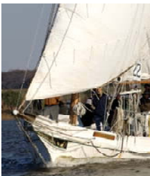
SKIPJACK ELSWORTH , Chestertown, Maryland Two-sailed bateau (skipjack), 72' sparred length, 18' beam, 23 gross tons Owner - Echo Hill Outdoor School, www.ehos.org
